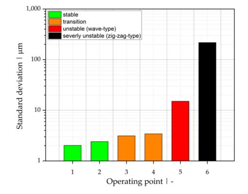
Process stability indicated by standard deviation of real depth position of the polymer-polymer interface
