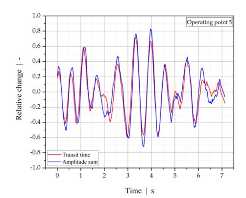
Relative change of transit time and amplitude (intensity) for US detection of flow instabilities
