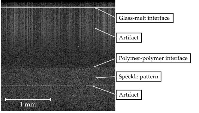
B-scan of OCT measurement during coextrusion showing glass-melt and polymerpolymer interfaces
