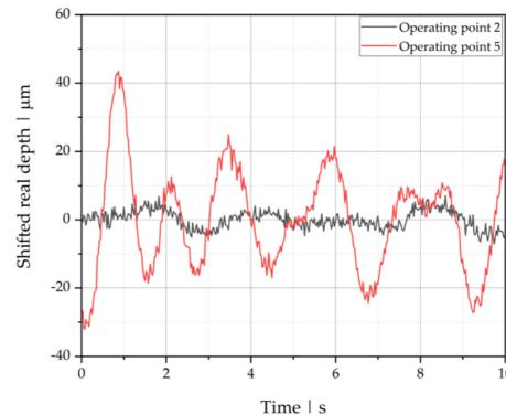
Real depth position of the polymer-polymer interface as function of time for an stable and unstable operating point
