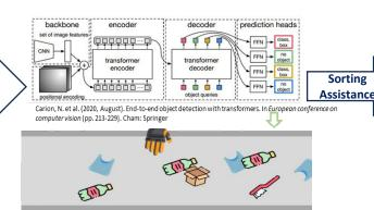
Neural networks (NN) are employed to detect the position of objects in the image. The NNs are fine-tuned and trained with custom data to fit the use case. However, deviations from the training environment can lead to outliers.
