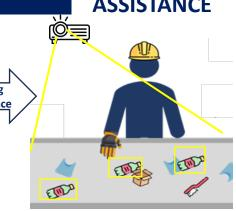
The visual waste assistance system supports workers during sorting tasks. Each item to be removed is highlighted with a segmentation mask or surrounded with borders, projected via a beamer based on the previous models.
