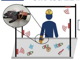
The glove's position is determined using Trilateration with (red) anchors attached to the corners of the sorting area. The 3D position of the glove is converted to the 2D coordinate system of the camera to be compared with the prediction of the neural network.
